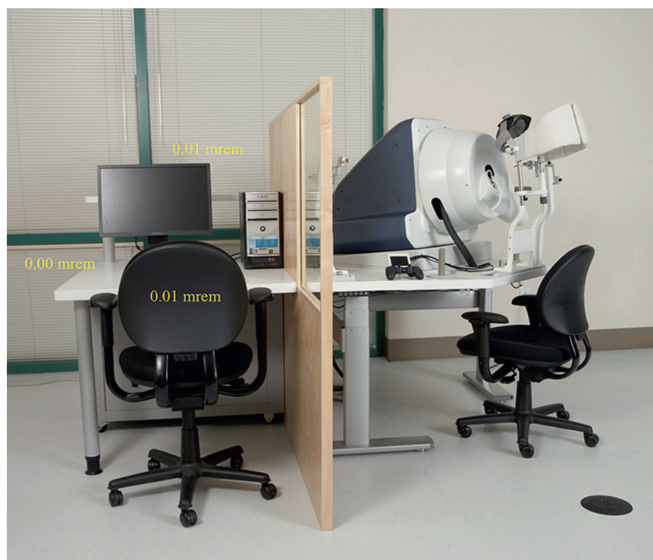
Figure 1 The clinical IRay device is shown. The operator console is to the left of a leaded glass shield. The patient is seated to the right of the leaded glass shield. The maximal radiation dose to the operator is 1 \times 10^{-7} Sv, equivalent to background radiation.
