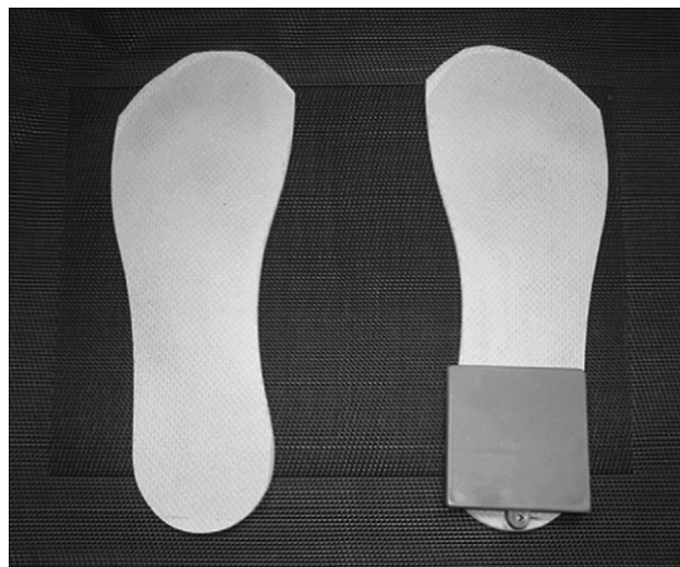
Figure 3 Photograph of foot plate with heel wedge inserted on the right foot.
